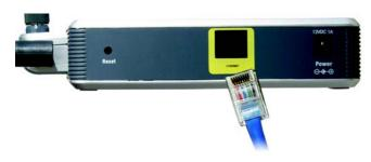
Figure 4-1: Connect the Ethernet Network Cable
